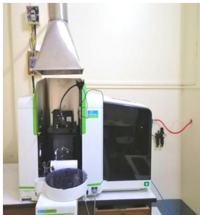
Figure 3 High-performance PinAAcle™ 900H atomic absorption spectrometer instrument in the laboratory of URC at Yangon University.
